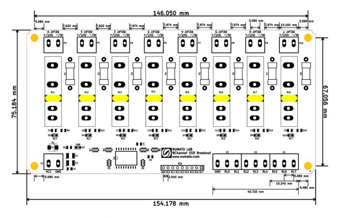
L x W x H : 154.178 mm x 75.184 mm x 30 mm Mechanical Hole Diameter- 4.0 mm
