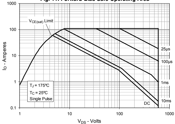
Fig. 11. Forward-Bias Safe Operating Area
