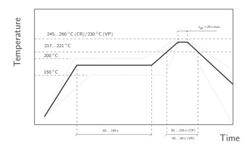
Recommended reflow soldering conditions following IPS/JEDEC J-STD-020.
