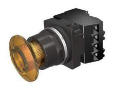
30mm BlackMax, Epoxy Coated Corrosion Resistant Complete Metal Unit Illuminated Twist-to-Release Full Voltage, 6V AC LED Lamp Mushroom Head Cap Small 1.79" (45 mm) Plastic Cap, Amber 2 Position Maintained, Twist-to-Release with 1 N.O. - 1 N.C. Heavy Duty Contacts, A600/P600 UL Listed, CSA Certified NEMA 1,3,3R,4,4X,12,13 & Automotive Standards
