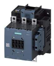
power contactor, AC-3e/AC-3 185 A, 90 kW / 400 V Uc: 24 V DC x (0.7-1.25) PLC input 24-110 V DC 3-pole, auxiliary contacts 2 NO + 2 NC drive: electronic main circuit: busbar control and auxiliary circuit: screw terminal extended rated condition railroad IEC 60077
