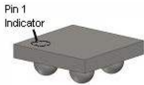
Figure 3. 1 x 1mm WLCSP Bumps Facing Down
