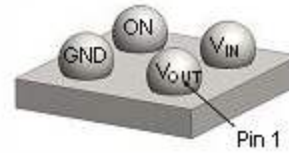
Figure 4. 1 x 1mm WLCSP Bumps Facing Up
