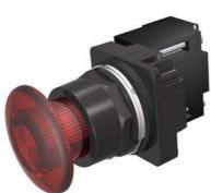
30mm BlackMax, Epoxy Coated Corrosion Resistant Complete Metal Unit Illuminated Push-Pull Operator Transformer type, 480V AC LED Lamp Mushroom Head Cap Small 1 3/4" (44.5 mm) Plastic, Red 2 Position Maintained, Pull-to-Release UL Listed, CSA Certified NEMA 1,3,3R,4,4X,12,13 & Automotive Standards
