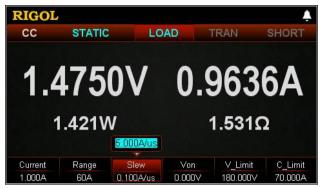
Current rising speed is defined as the speed of transition from one setting to another. You can set the actual transition time from one setting to another by changing the current rising speed. Adjustable current rising speed: 0.001 A/ $\mu$ s to 5 A/ $\mu$ s.
