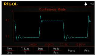
The electronic load provides the waveform display function and supports the following operations for the waveform, such as pausing the waveform, recording the waveform, and capturing the waveform. Therefore, you can dynamically observe the trend of parameters changes.
