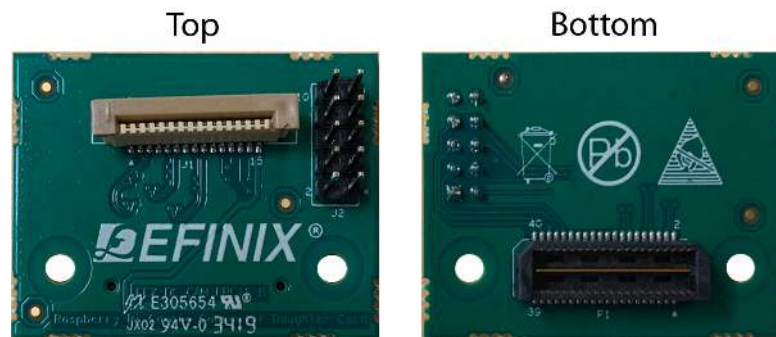
Figure 5: Raspberry Pi Camera Connector Daughter Card
