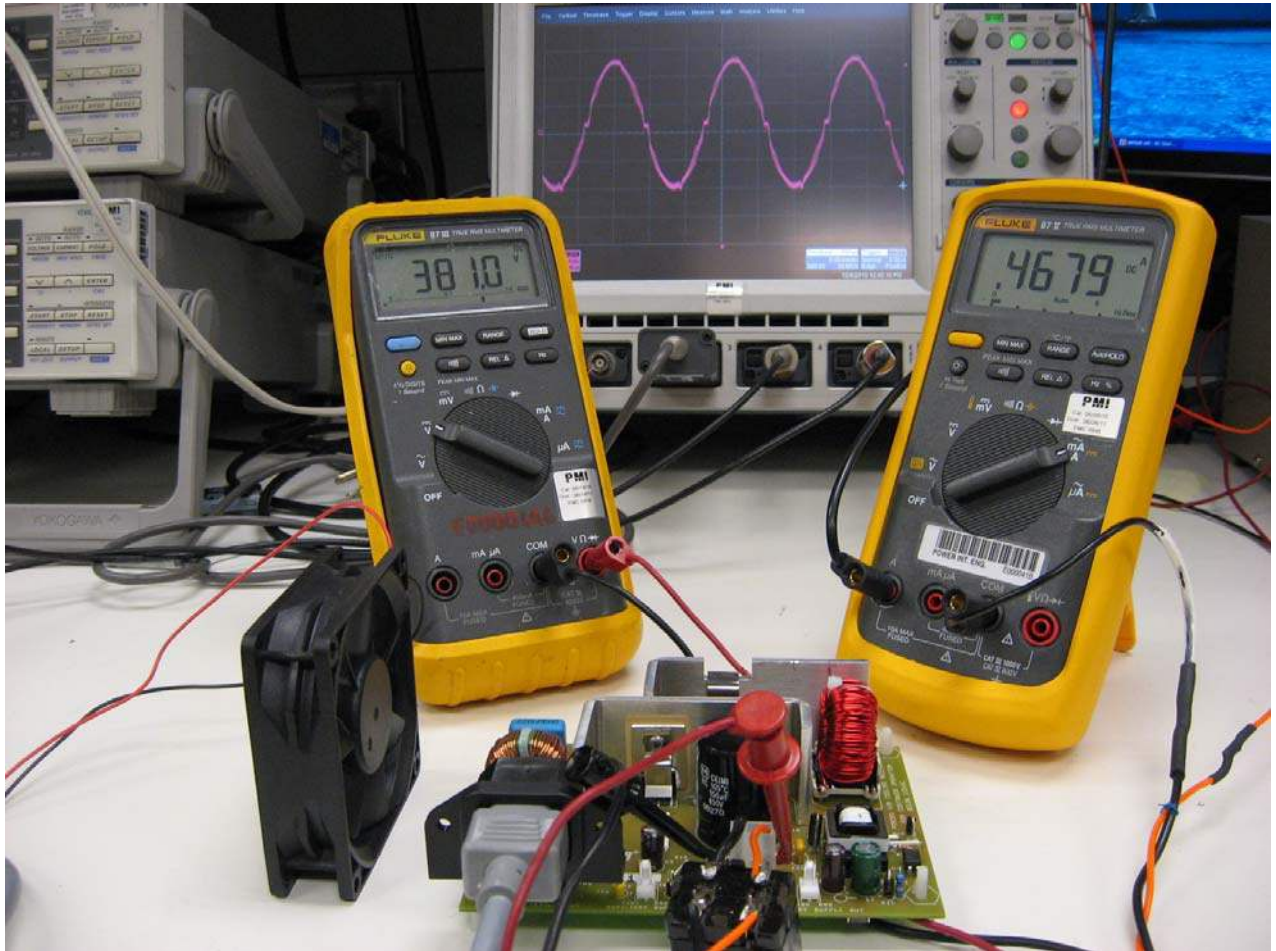
Figure 83 – Front View of the Test Set-up for Efficiency, PF and THDi Measurements.
