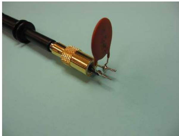
Figure 67 – Oscilloscope Probe with Probe Master ( www.probemaster.com ) 4987A BNC Adapter (Modified with wires for ripple measurement, and one parallel decoupling capacitor added.)
