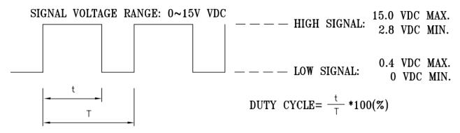
\*THE FREQUENCY FOR CONTROL SIGNAL OF THE FAN SHALL BE ABLE TO ACCEPT 600HZ~30KHZ WITH DIFFERENT SPEED PERFORMANCE.
