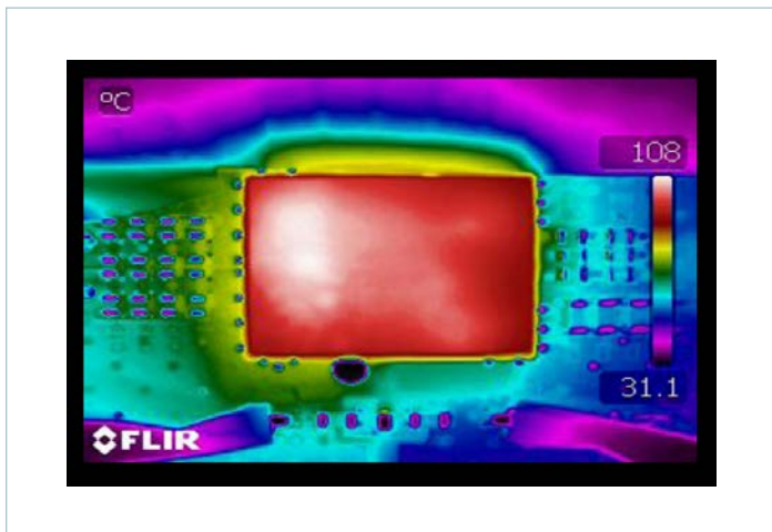
Figure 10 — Thermal image ( V_{IN} = 48V , I_{OUT} = 18A , CR, OLFM evaluation PCB)
