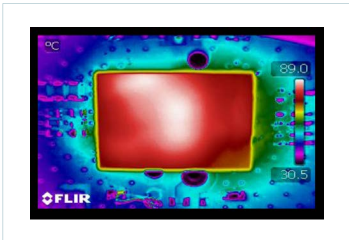
Figure 20 — Thermal image ( V_{IN} = 48V , I_{OUT} = 5A , CR, OLFM evaluation PCB)
