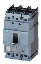
circuit breaker 3VA5 UL frame 125 breaking capacity class S 25kA @ 480 V 3-pole, line protection TM230, FTAM, In=100A overload protection Ir=100A fixed short-circuit protection Ii=5...10 x In UL489 SB (naval), 50 deg. cel. cable connection on both sides
