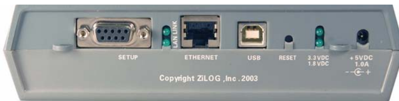
Figure 3. Crimzon ICE Rear Panel
