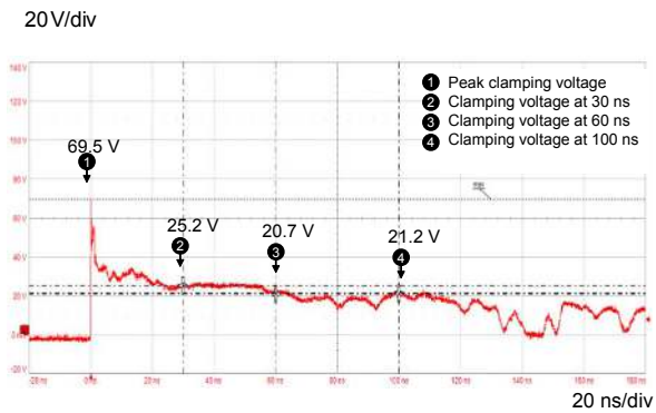
Figure 5. ESD response to IEC 61000-4-2 (+8 kV contact discharge)
