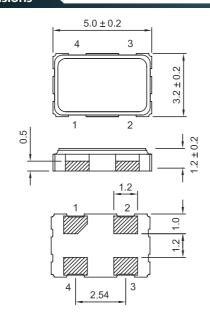
PAD FUNCTION: 1:ENABLE CONTROL 2:GND 3:OUT 4:VDD
