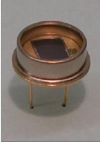
PACKAGE DIMENSIONS INCH [mm] 0.215 [5.46] Ø0.483 [12.27]-- 0.065 [1.65] WIRE BONDS Ø0.449 [11.39] 1.50 [38.1] Ø0.55 VIEWING 0.295 [7.49] ANODE ANGLE Ø0.018 [0.46] CATHODE Ø0.018 [0.46] -HEADER PHOTODIODE OUARTZ WINDOW CAP (WELDED) 0.340 [8.64] 0.209 [5.31] ACTIVE AREA 0.230 [5.84] TO-8 PACKAGE - 0.319 [8.10] ACTIVE AREA ACTIVE AREA = 42.86 mm<sup>2</sup>
