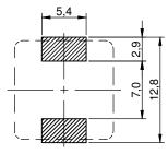
no vias and sensitive traces underneath the component Scale - 2:1
