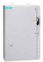
Non-reversing motor starter, Size 2 1/2, Three phase full voltage, Solid-state overload relay, OLRelay amp range 25-100A, 190 220/220 240V 50/60HZ coil, Combination type, 100A non-fusible disconnect, Enclosure NEMA type 4/12, Water/dust tight for outdoors, Standard width enclosure
