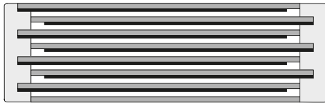
Extended metallized film design
