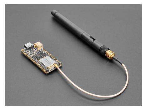
Your Feather Radio does not have a built-in antenna. Instead, you have two options for attaching an antenna. For most low cost radio nodes, a short length of wire works
