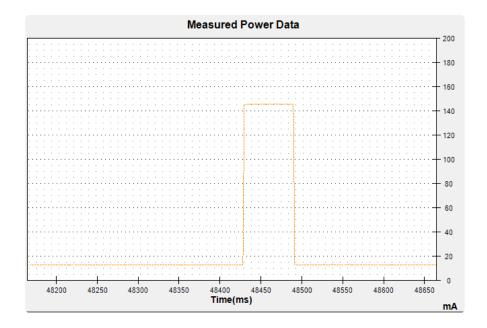
The ~13mA quiescent current is the current draw for listening (~2mA) plus ~11mA for the microcontroller. This can be reduce to amost nothing with proper sleep modes and not putting the module in active listen mode!
