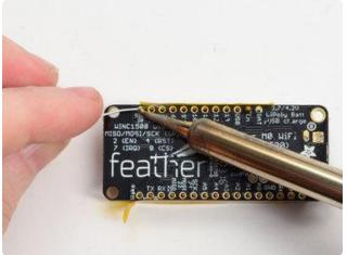
Flip & Tack Solder After flipping over, solder one or two points on each strip, to 'tack' the header in
