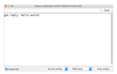
To receive a message simply call the **receive** function. This function will wait for half a second for any packet to be received. If a packet is found it will be returned as a byte string (remember packets are at most 252 bytes long), or if no packet was found a result of **None** is returned.
