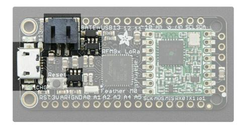
The above shows the Micro USB jack (left), LiPoly JST jack (top left), as well as the 3.3V regulator and changeover diode (just to the right of the JST jack) and the LiPoly charging circuitry (to the right of the Reset button).
