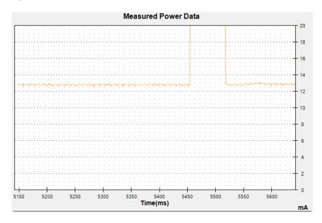
You can put the module into sleep mode by calling radio.sleep(); which will save
