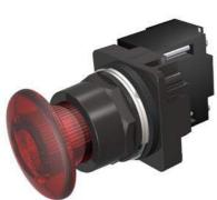
30mm BlackMax, Epoxy Coated Corrosion Resistant Complete Metal Unit Illuminated Push-Pull Operator Full Voltage, 120V AC/DC Incandescent Lamp Mushroom Head Cap Small 1 3/4" (44.5 mm) Plastic, Red 2 Position Maintained, Pull-to-Release UL Listed, CSA Certified NEMA 1,3,3R,4,4X,12,13 & Automotive Standards
