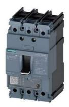
circuit breaker 3VA5 UL frame 125 3-pole, starter protection TM120M, AM, In=125A without overload protection short-circuit protection Ii=5...12 x In nut keeper kit on both sides
