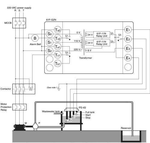
**Automatic Drainage Control with Abnormal Water Increase Alarm**
