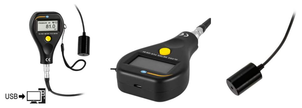
Gloss meter with external gloss sensor / Measurement geometry 60° / Measuring surface Ø4.5 mm Data connection with a PC via micro USB interface / One button operation / Calibration standard included / Data storage for 1245 measurements
