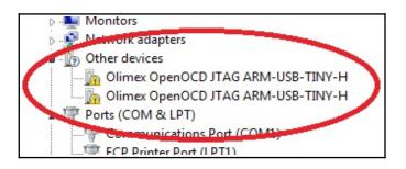
The driver installation in Windows would depend on which version of OpenOCD you are using. There is a difference in the driver installation if you are using OpenOCD 0.8.0 or newer and if you are using versions prior to OpenOCD 0.8.0.
