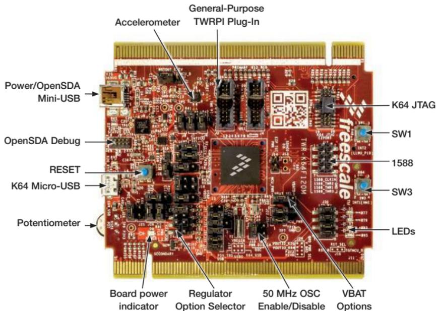
Figure 1: Front side of TWR-K64F120M
