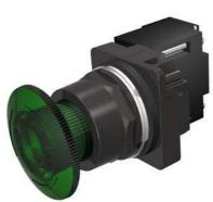
30mm BlackMax, Epoxy Coated Corrosion Resistant Metal Operator, Round Illuminated Twist-to-Release Transformer type, 480V AC LED Lamp Mushroom Head Cap Small 1.79" (45 mm) Plastic Cap, Green 2 Position Maintained, Twist-to-Release UL Listed, CSA Certified NEMA 1,3,3R,4,4X,12,13 & Automotive Standards
