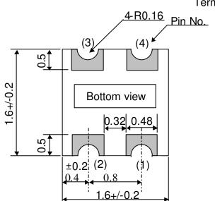
[Recommended PCB pad dimensions] Unit: mm
