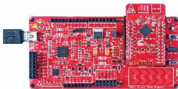
Fig-3: Programming and Debugging with CY8CKIT-042-BLE Pioneer Baseboard
