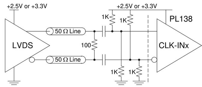
This circuit is for compatibility only. AC coupling is not really required for LVDS. The  $V_{CMR}$  range of the PL138 reaches low enough that LVDS signals can be connected directly to the PL138 input like in the circuit to the left.
