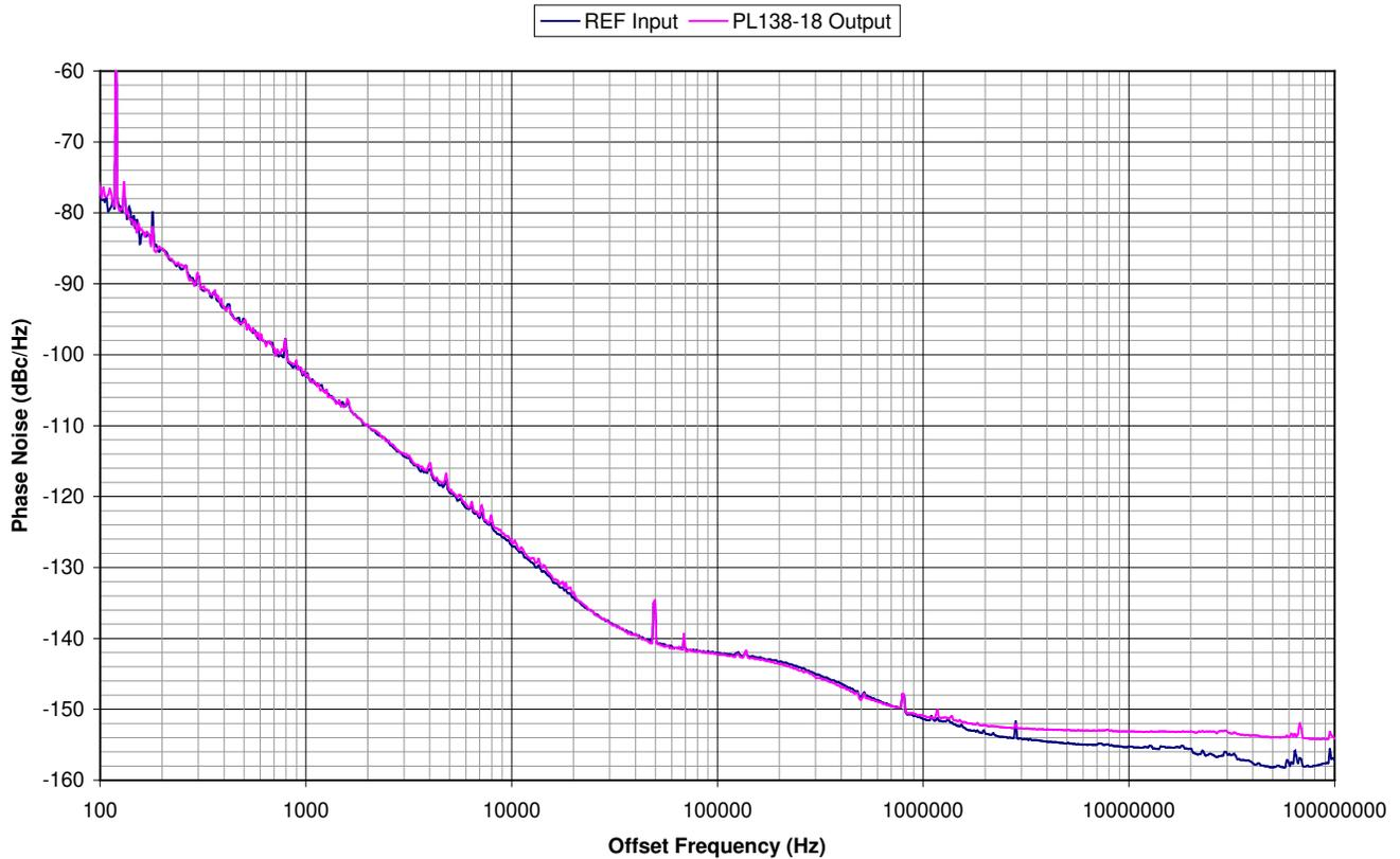
When a buffer is used to pass a signal then the buffer will add a little bit of its own noise. The phase noise on the output of the buffer will be a little bit more than the phase noise in the input signal. To quantify the noise addition in the buffer we compare the Phase Jitter numbers from the input and the output. The difference is called "Additive Phase Jitter". The formula for the Additive Phase Jitter is as follows:
