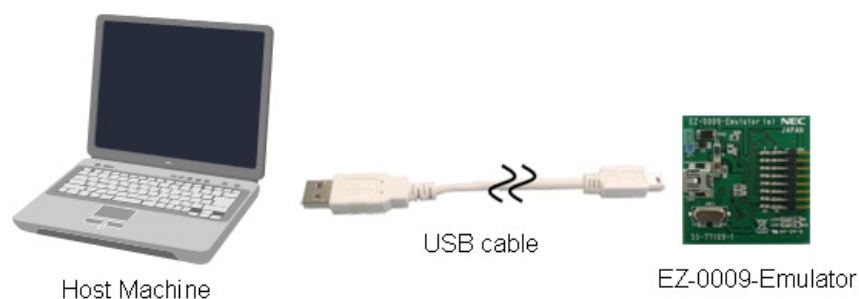
Figure3-8 Connecting EZ-0009-Emulator to Host machine
