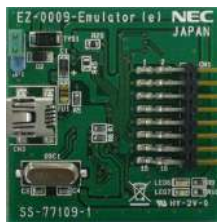
Simple On-chip debug emulator (EZ-0009-Emulator)
