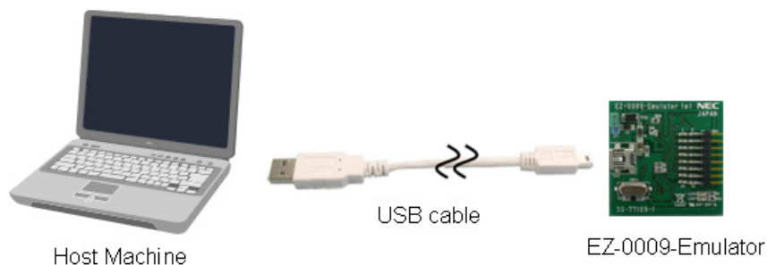
Figure3-5 Connecting EZ-0009-Emulator to Host machine
