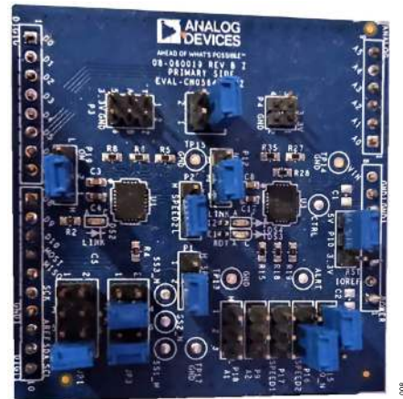
Figure 8. Jumper Configurations on the Local and Remote LTC4332
