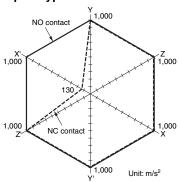
Sample: G2RL-14 12 VDC Number of relays: 5 pcs Test conditions: Shock is applied in  $\pm X$ ,  $\pm Y$ , and  $\pm Z$  directions three times each with without energizing
