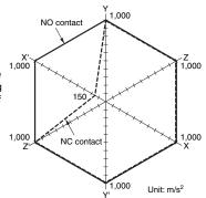
Sample: G2RL-24 12 VDC Number of relays: 5 pcs Test conditions: Shock is applied in  $\pm X$ ,  $\pm Y$ , and  $\pm Z$  directions three times each with without energizing the Relays to check the number of
