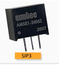
Aimtec's AMSR1-Z is a 1A Switching Regulator which is designed to be a plug and play alternative to the traditional 78xx series three-terminal linear regulators. The series features an ultra-wide input voltage range of 4.6-36V, 1.5mA ultra- low no load input current, continuous short-circuit protection, low ripple noise (max.: up to 50mV) and much more.
