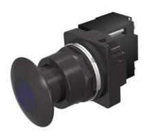
30mm BlackMax, Epoxy Coated Corrosion Resistant Complete Metal Unit Illuminated Push-Pull Operator Transformer type, 600V AC LED Lamp Mushroom Head Cap Small 1 3/4" (44.5 mm) Metal, Black with Blue Lens 2 Position Maintained, Pull-to-Release UL Listed, CSA Certified NEMA 1,3,3R,4,4X,12,13 & Automotive Standards
