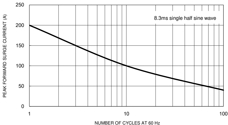
Fig.5 Maximum Non-Repetitive Forward Surge Current
