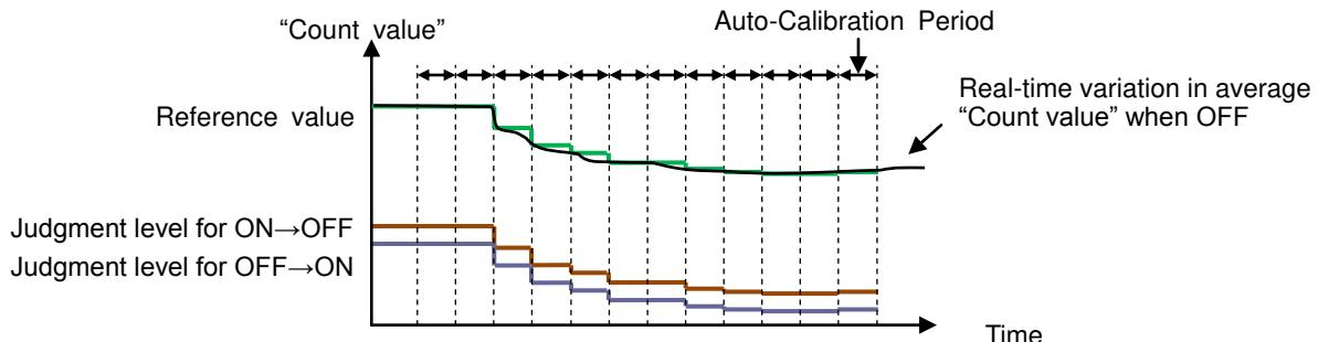
\*: The “Reference value” will re-adjust each Auto-calibration period. The “Threshold value” and the “Hysteresis value” are relative values, so each “Judgment level” for ON/OFF will continue to remain at the same relative level, in synchronization with the “Reference value”.
