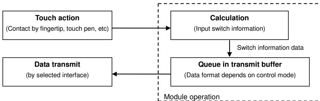
Note: Switch status information can be sent to the host in response to a touch status read command, or it can be sent automatically whenever touch status changes. Current touch status can also be read within a Program Macro, and via the Key Scan interface (if Key Scan mode is enabled).
