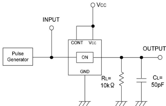
Note: Open output when measuring supply current
