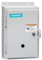
Reversing contactor Size 1 3/4 Three phase full voltage Contactor amp rating 40Amp 3 w 110V 50HZ / 120V 60HZ coil Non-combination type Enclosure NEMA type 12 Dust/drip proof for indoors Standard width enclosure
