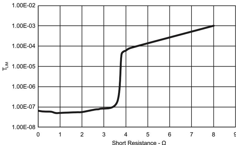
Figure 8. Overcurrent Response Time vs Short Resistance
