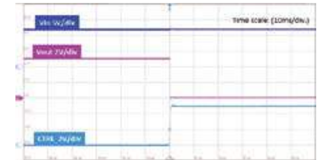
Figure 9: CNTL high level, DC-DC off
