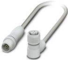
Sensor/Actuator cable, 5-position, PP-EPDM halogen-free, Gray RAL 7035, Plug straight M12, A-coded, on Socket angled M12, A-coded, with 3 LEDs, Cable length: 0.3 m, Hygienic design, with plastic knurl
