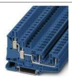
Feed-through terminal block, Connection method: Pluggable screw terminal block, Cross section: 0.2 mm² - 10 mm², AWG: 24 - 8, Width: 8.2 mm, Color: blue, Mounting type: NS 35/7,5, NS 35/15
