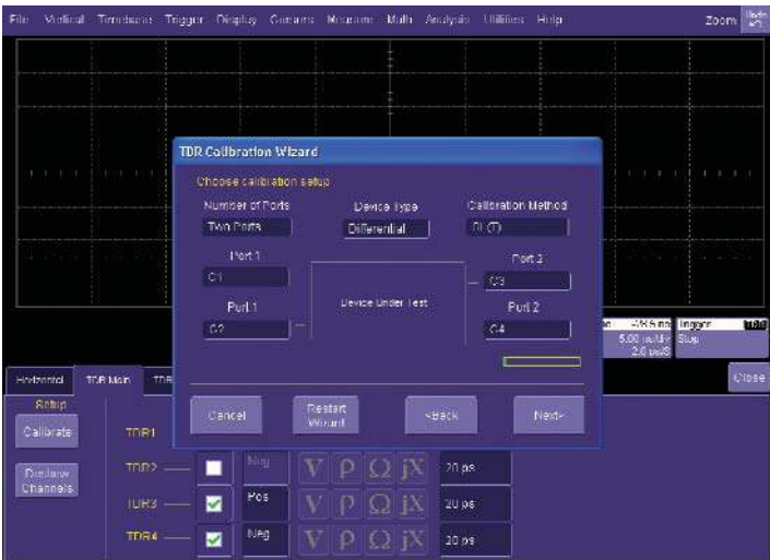
The TDR measurement wizard guides the user through the set-up and calibration process ensuring the highest accuracy measurements. Full reference plane calibration and channel deskew is performed by the wizard.
