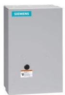
Electrically held lighting contactor, Contactor amp rating 30A, 0 N.C. / 6 N.O. Poles, 600VAC 60HZ coil, Non-combination type, (no disconnect device), Enclosure NEMA type 1, Indoor general purpose use
