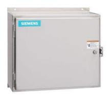
Mechanically held lighting contactor, Contactor amp rating 30Amp 0NC  $\_$  12NO poles, 208VAC 60HZ coil, Non-combination type, Enclosure NEMA type 12, Dust/drip proof for indoors
