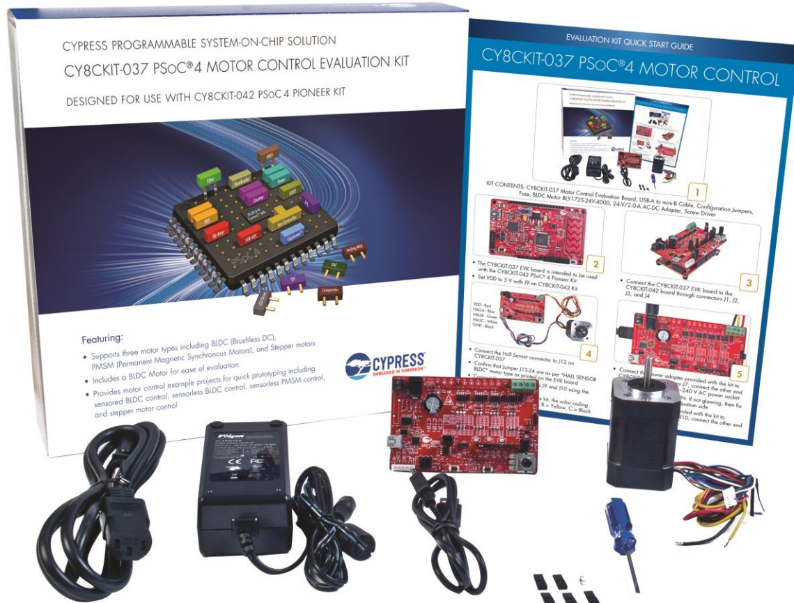
Figure 1-1. CY8CKIT-037 PSoC 4 Motor Control EVK Contents
