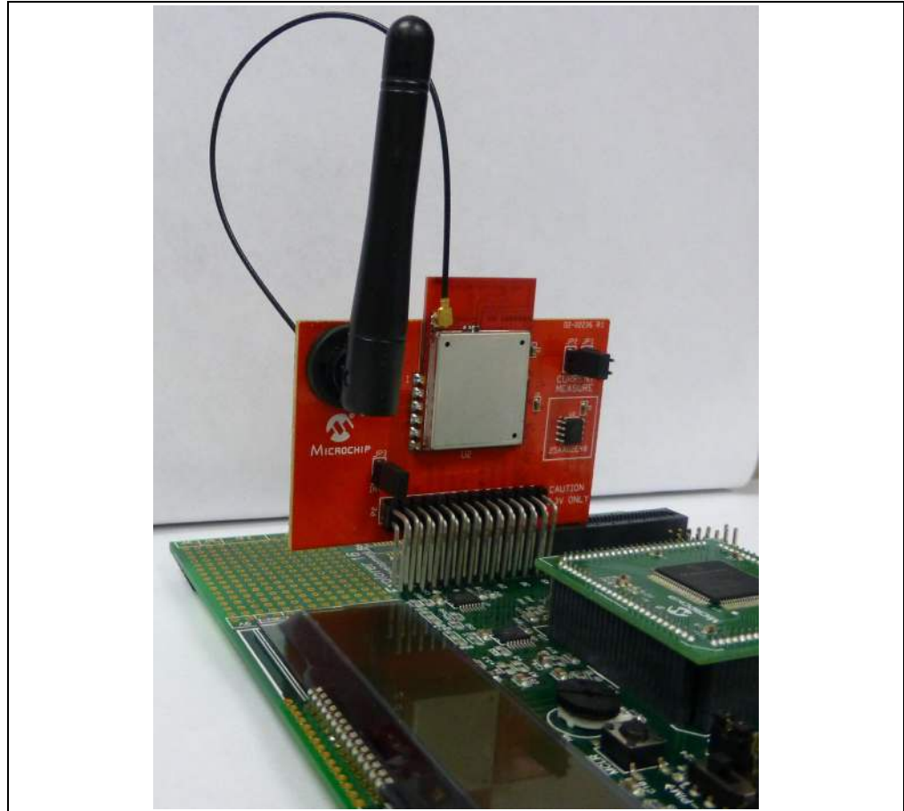
FIGURE 2-2: MRF24J40ME PICtail™/ PICtail Plus Daughter Board PLUGGED INTO EXPLORER 16 DEVELOPMENT BOARD
