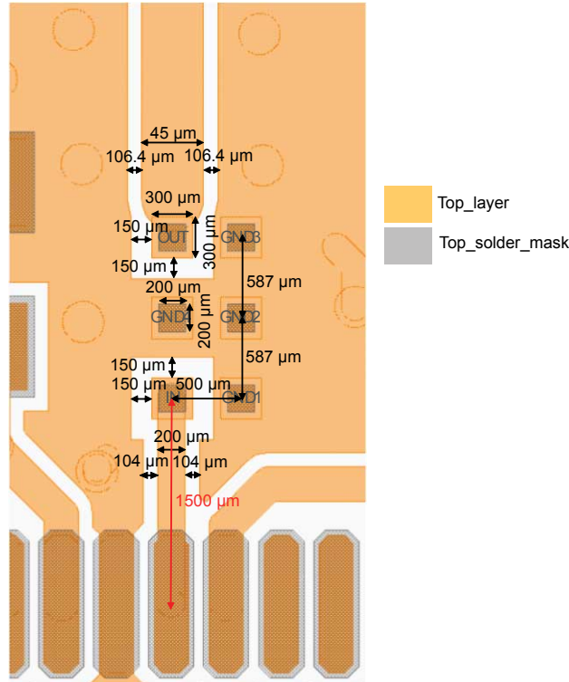
Figure 13. PCB land pattern recommendations
